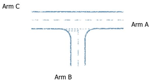
Table 4.2 shows case study results comparing **fast-answers quick-PJ** with TRL's Picady. The main carriageway has a width of 8m and observations on site have shown there is insufficient space for ahead traffic to pass right turners waiting to turn (drive on left system). These right turners subsequently block the road for ahead traffic.
